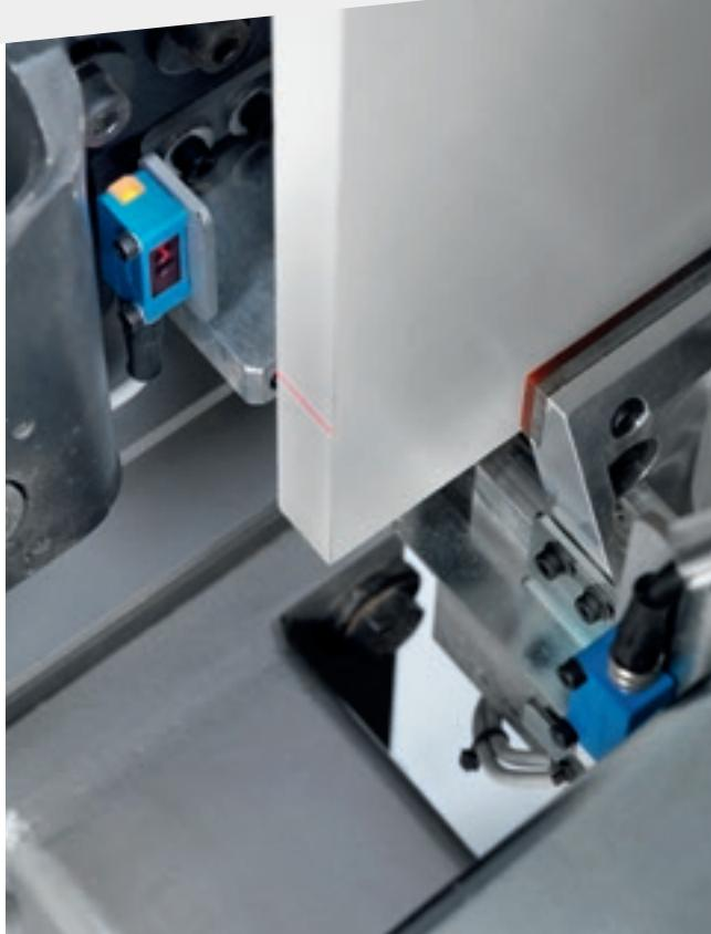
The **laser scanner** system that detects the start and the end of the panel enables the machine to compensate dimensional errors, correcting the panel's X dimensions.
