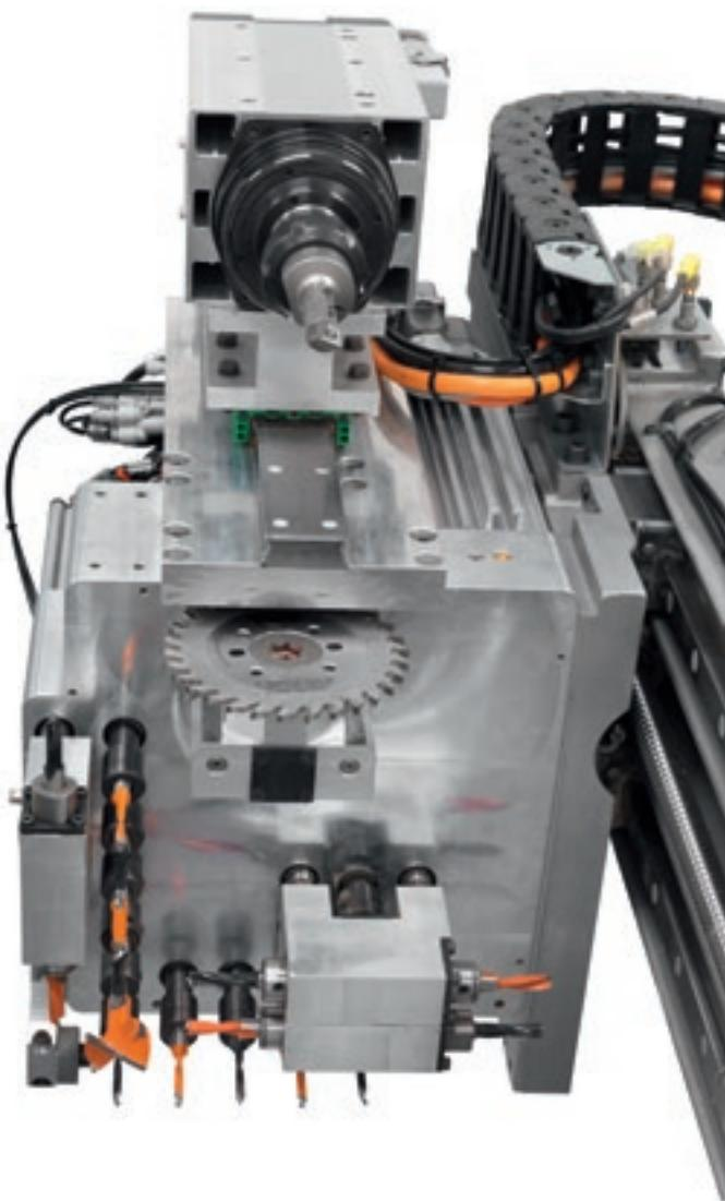
Milling units from 4.5 to 5.5 kW and drilling units with 17 or 23 tools are available.
