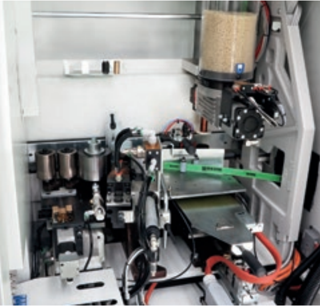
Gluing unit for the automatic application of edging in rolls or strips, from 0.4 to 12mm.
