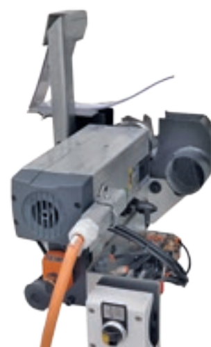
The Grooving Unit creates grooves and performs milling operations on the underside of the panel.
